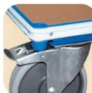
Protective strip made of plastic profile, attached around the basic frame. Protects door frames and walls from damage, scratches etc. Cannot be retrofitted
